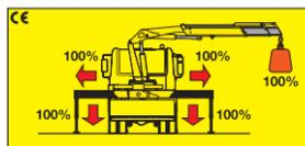
The **HM System** integrated in the load limiting device checks the stabilizers' positions. Only when all beams are fully open and all stabilizers are on the ground the crane can operate and lift loads.
