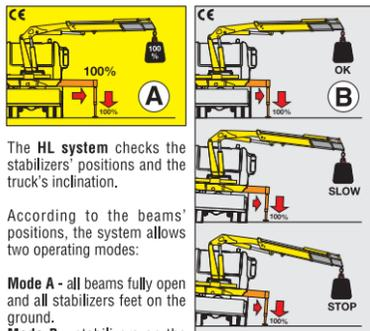
In **mode A**: the load limiting device stops the crane when the crane reaches 100% of the nominal capacity.
