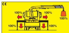
The **HML System** integrated in the load limiting device checks the stabilizers' positions. Only when all beams are fully open and all stabilizers are on the ground the crane can operate and lift loads.
