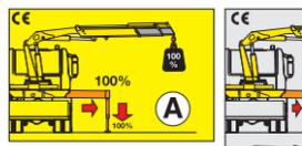
The HL system checks the stabilizers' positions and the truck's inclination.
