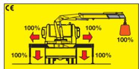
The HML System integrated in the load limiting device checks the stabilizers' positions. Only when all beams are fully open and all stabilizers are on the ground the crane can operate and lift loads.
