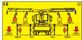
The TCU checks the positions of the stabilizers beams, monitoring for two possible positions: beam fully open, beam not fully open. Depending on the position of the beams and the stabilizers, the crane's lifting capacity changes according to the setting made by the installer. This allows the operator to use the crane even with a beam partially or fully retracted without having stability problems.
